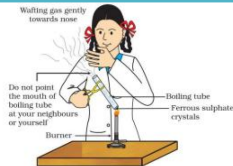
Correct way of heating the boiling tube containing crystals of ferrous sulphate and of smelling the odour
