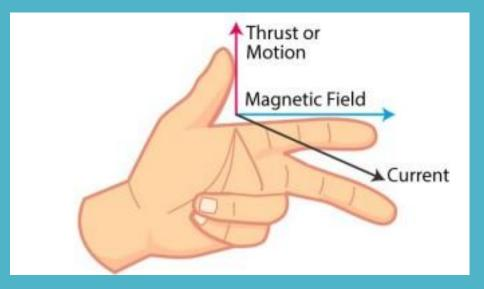
Force on a Current-carrying Conductor in a Magnetic Field
