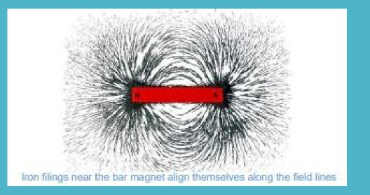
• The direction of the magnetic field at any point is obtained by drawing a tangent to the field line at that point.
