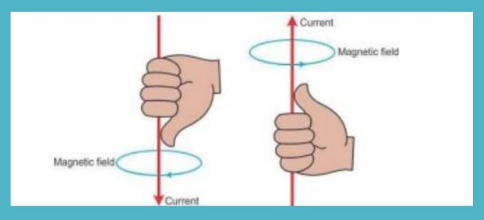
Magnetic Field due to a Straight Current-carrying Conductor
