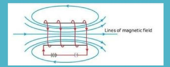
Magnetic Field due to a Current-carrying Solenoid
