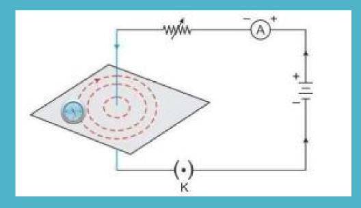
Magnetic Field due to a Straight Current-carrying Conductor
