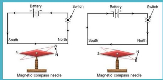
Magnetic Field due to a Straight Current-carrying Conductor
